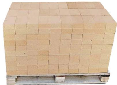
Vitcas® Firebricks are High Duty Fireclay bricks with a low iron and alkali content. The maximum temperature in service is 1430°C/2600°F and the density is 2200kg/m<sup>3</sup>. Dense firebricks are preferred where higher thermal mass and heat storage are important.
