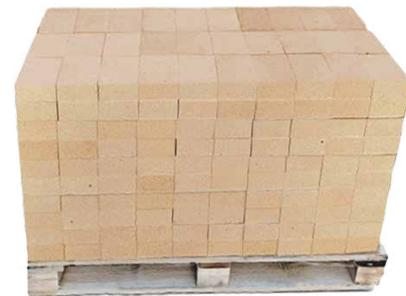
Vitcas High Alumina Bricks have a high density and high strength. The maximum temperature in service is 1450°C 2640°F with a density of 2600kg/m<sup>3</sup> and an alumina content of 60%.
