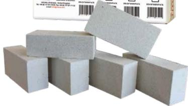
The Vitcas® range of Insulation Firebricks are made from specially formulated high-purity refractory clays with varying alumina contents in a manufacturing process which results in a controlled pore structure. They are much less dense and therefore lighter in weight than fireclay bricks. The low thermal mass makes them most suitable for situations where heat storage is to be avoided.
